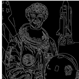
Edge Detection (Canny, \sigma = 1 )
